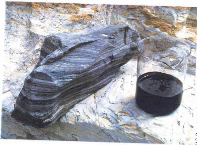
Figure 15-7 Heavy shale oil (right) can be extracted from oil shale rock (left).
