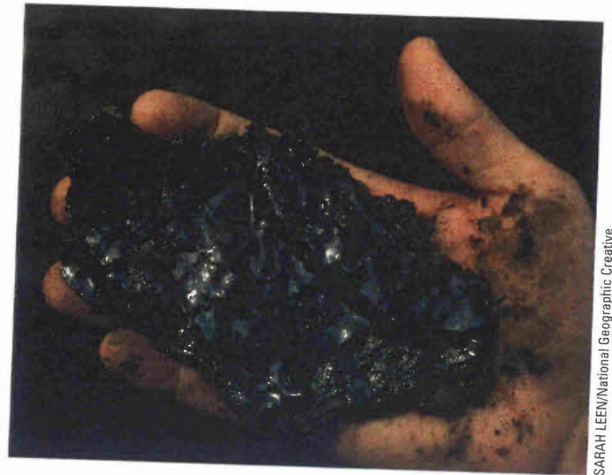
Figure 15-8 This gooey tar, or bitumen, with the consistency of peanut butter, was extracted from tar sands in Alberta, Canada, to be converted to heavy synthetic oil.
